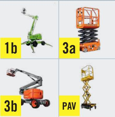
**1b** Static boom access platform (unable to move elevated, requires outriggers)
