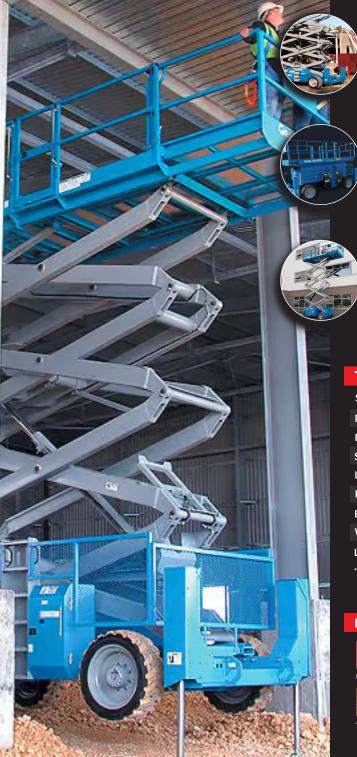
Active Oscillating axle keeps the wheels on the ground during operation
