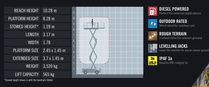
The Haulotte Compact 10DX diesel scissor lift has 4 wheel drive and rough terrain tyres and is perfect for working on construction sites. Hydraulic outriggers keep the platform stable while the extending platform provides over 5.3 square metres of usable platform that can lift several operators and equipment with ease.
