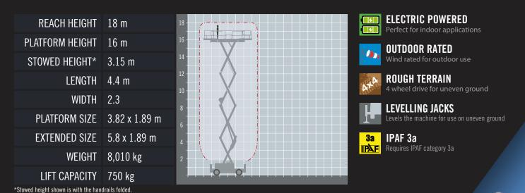
The Haulotte HS18E Pro is a 4 wheel drive rough terrain electric/hybrid scissor lift. With a working height of 18 metres, a platform that extends to almoist 6 metres and a platform capacity of 750kg this scissor lift provides ample working space for 4 people and their tools. An optional 'Range Extender' diesel power pack is also available which allows the machine to be operated while being charged.
