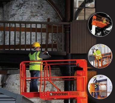
Self Propelled compact vertical mast lift
