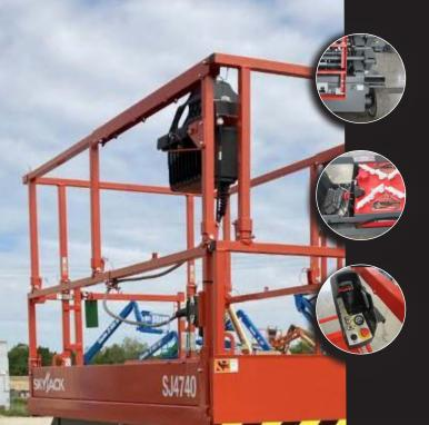
13.86 meters reach height Up to 25% Gradeability 28 mph wind rating (12.5 m/s) Forklift pockets & tie down\lift lugs
